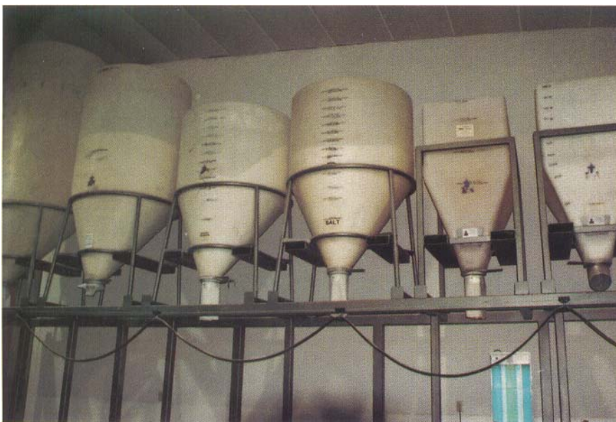
Ingredient levels can be viewed through the polyethylene bins.
