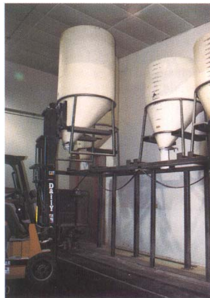
The bins are moved from the frame to the floor for filling.
