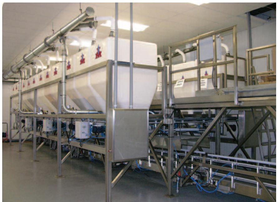
The automated weighing and batching system can make a spice batch with up to 24 different ingredients in less than 8 minutes.
