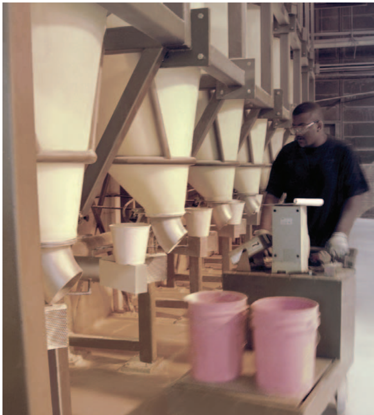
Tyrolit uses a bulk bag system, manufactured by Ingredient Masters, to optimize the handling of powdered ingredients used in vitrified bonds at their Cincinnati facility. Above, an operator meters product from 70 cu. ft. bins on Tyrolit's major ingredient line.
